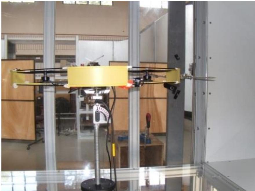
**Figure 5: Quadrotor with load cell and RPM Sensor**
