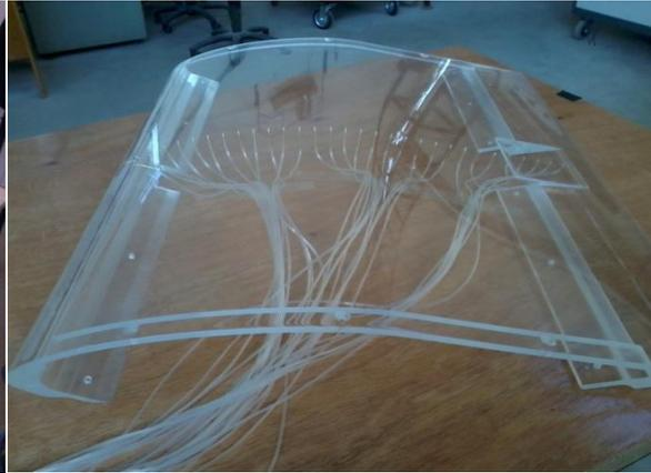
Figure 3. Detachable part with pressure taps
