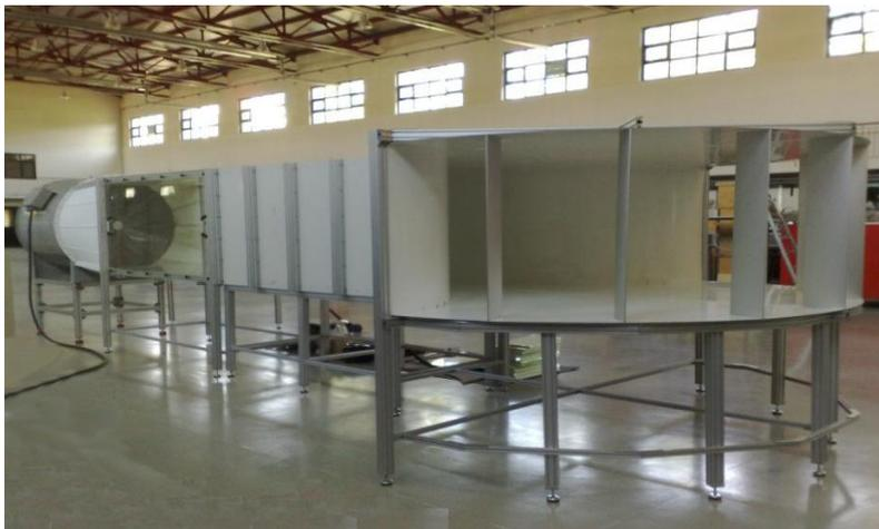
Figure1. Picture of METUWIND's suction type wind tunnel that has a 1 m x 1 m test section area.
