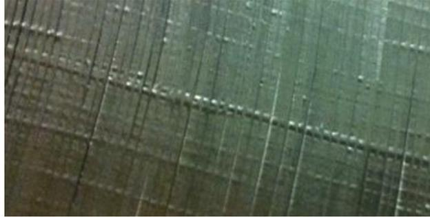
**Figure 8** Local fiber buckling
