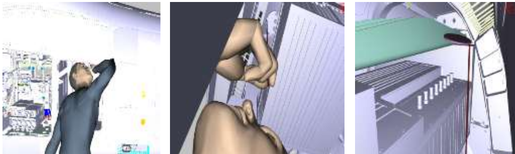
Figure 3: Digital Mock-Up for Inspection of an Equipment Using a Mirror by Maintenance Person [1].
