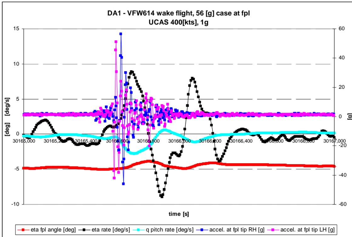
Figure 19: Foreplane angle and rate; acceleration of foreplane tip LH/RH
