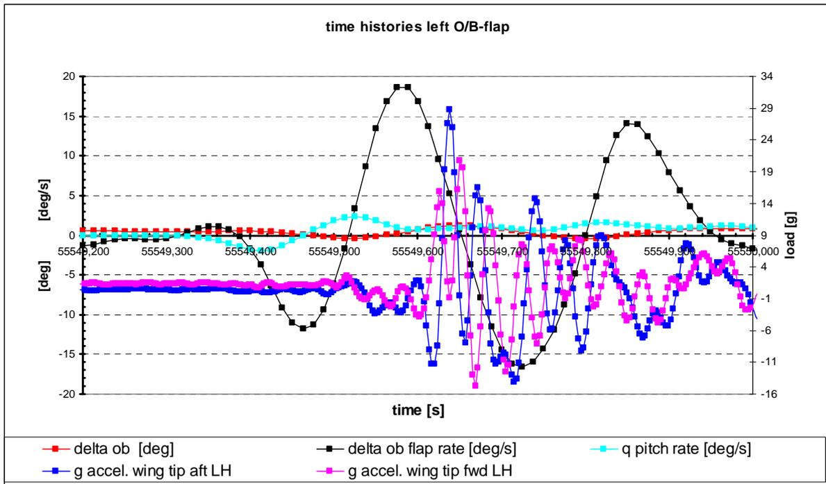
Figure 13: Left O/B flap angles and rate; q and acceleration of fwd wing tip
