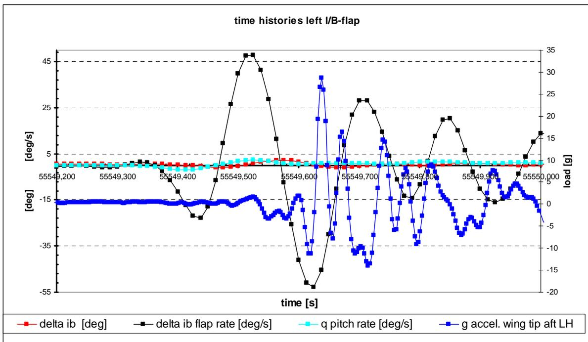
Figure 14: Left I/B flap angles and rate; q and acceleration of aft wing tip
