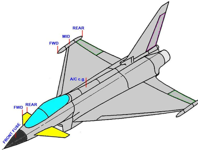
Figure 10: Accelerometer installation for flight test
