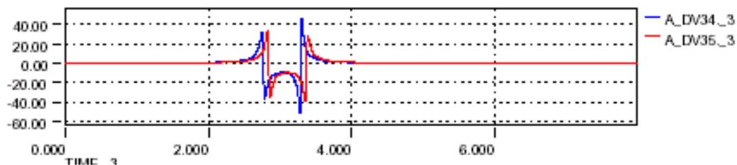
Figure 8: *Airbus A310 wake prediction max vertical velocity 42 m/s; generating aircraft A310 Speed: 325 KCAS*
