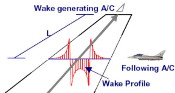
Figure 5: Wake profile from wake generating aircraft, from Ref. 11
