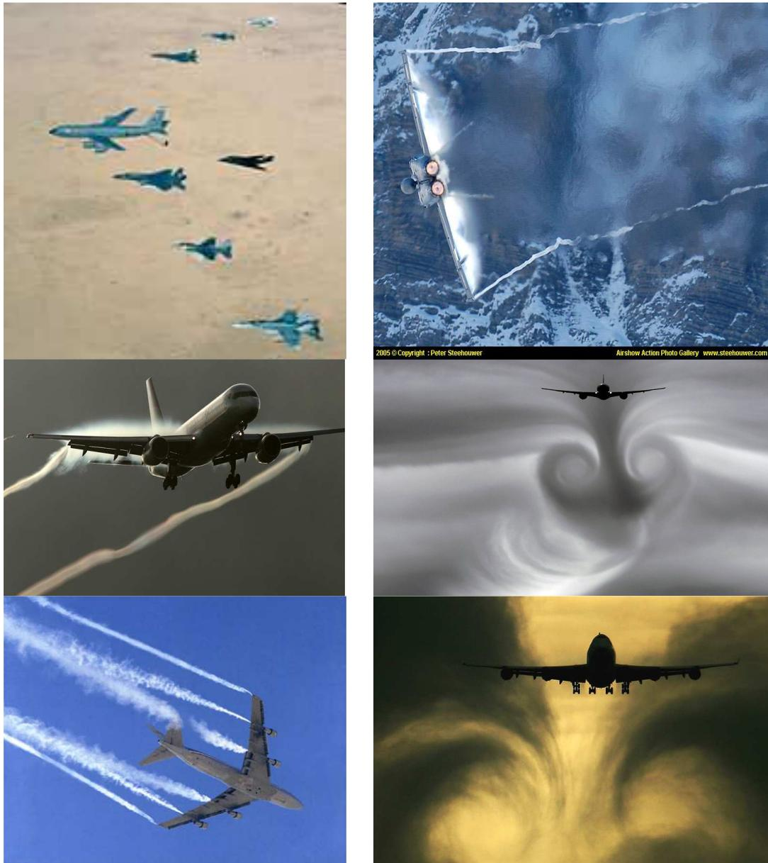
Figure 1: Formation flight and maneuvering of military aircraft and vortex generation by different transport aircraft – Boeing 757, 777, 747, Ref. 10
