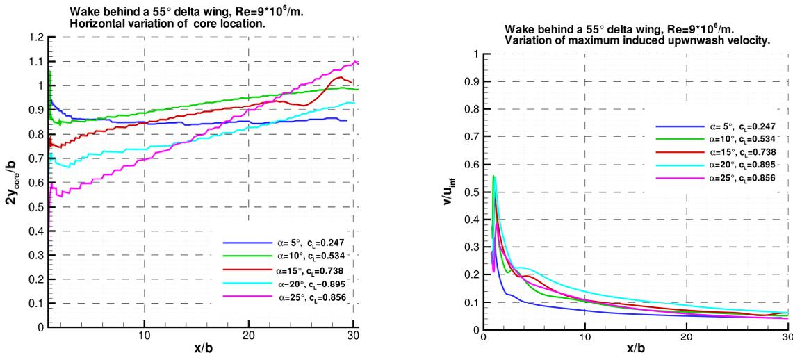
Figure 20: Wake velocity behind Fighter
