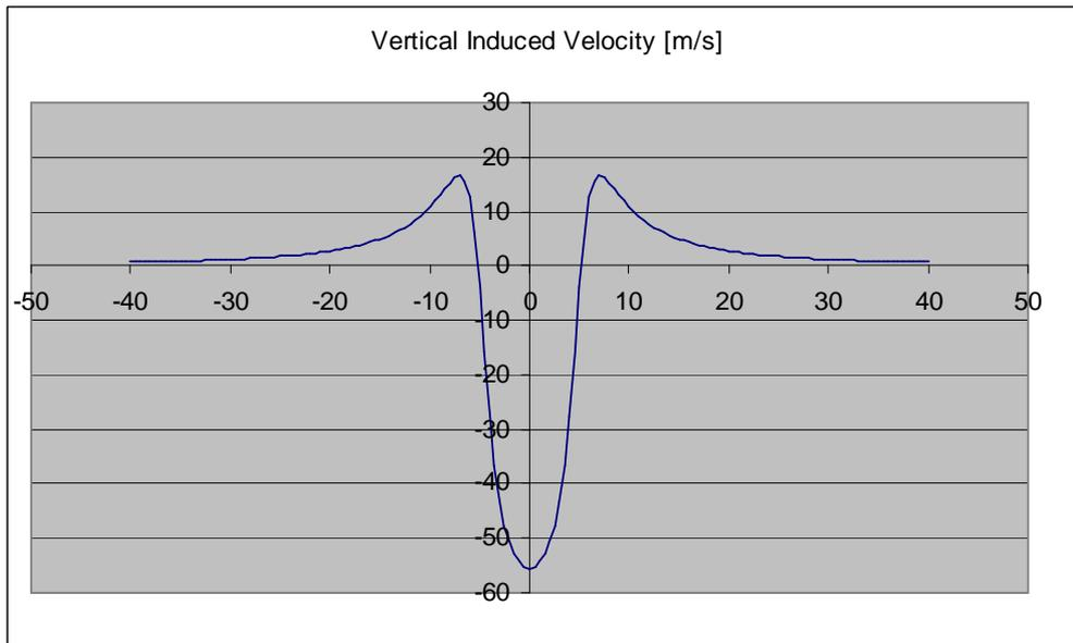
Figure 7: Calculated wake generation by Fighter Aircraft 350 KCAS, 20 deg. AoA; 10 000 ft a distance of 800 ft for further dynamic response calculation of flexible A/C
