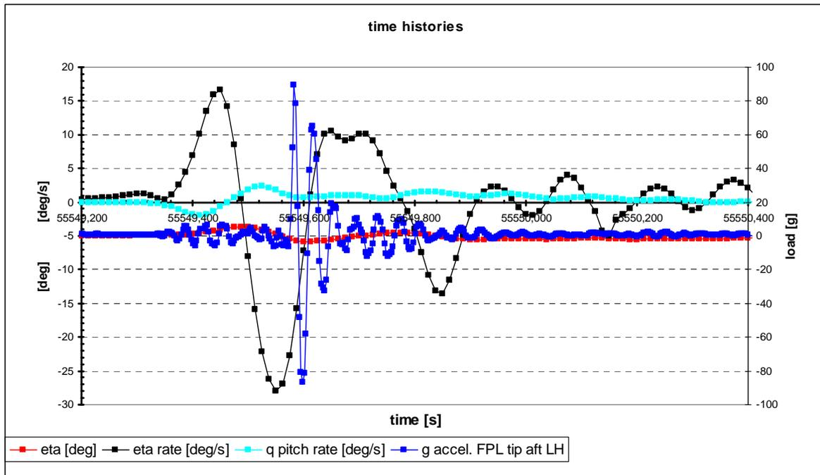
Figure 15: Left foreplane angle and rate; acceleration of foreplane tip;
