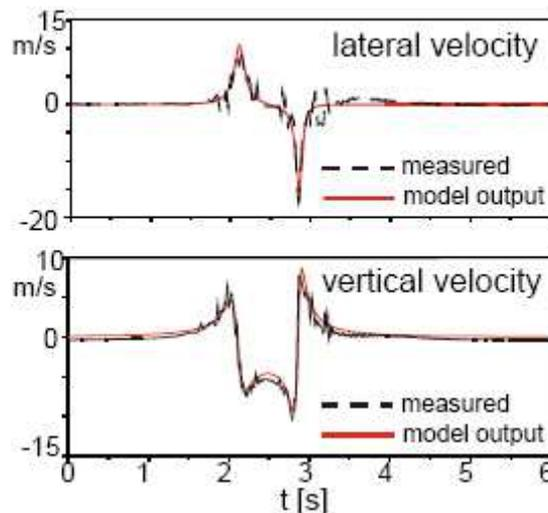
Figure 3: Vortex induced velocity distribution, from Ref. 2
