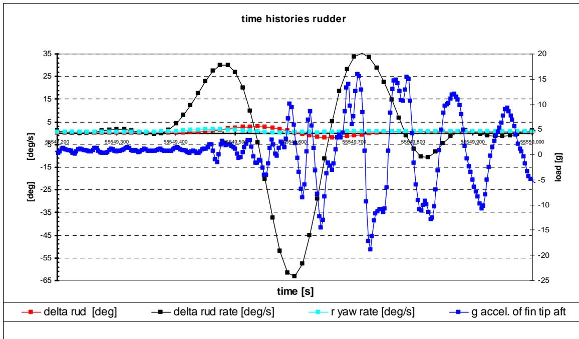
Figure 17: Rudder angle and rate; acceleration of fin tip
