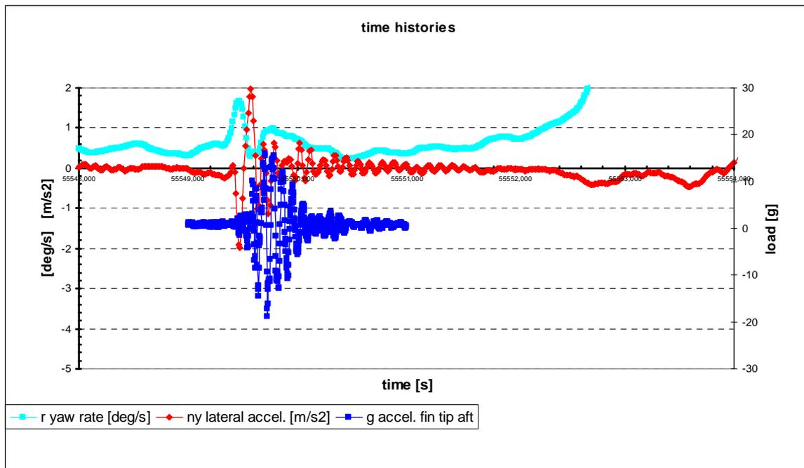
Figure 18: Time history of yaw rate, lateral  $n_y$  and acceleration of fin tip due Fighter wake
