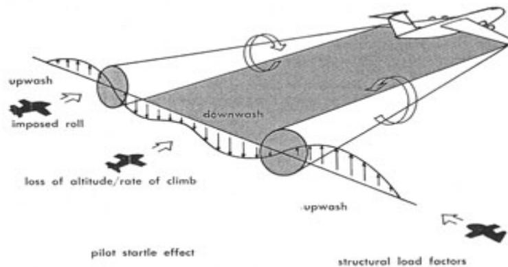
Figure 4: Wake profile behind generating aircraft (Ref. 9)
