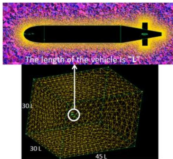
Figure 8: *Grids of Fluid Domain of Autosub AUV.*
