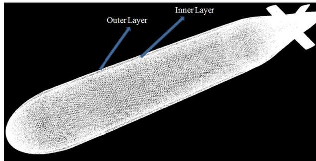
Figure 7: *Structure of Boundary Layers of Autosub AUV.*
