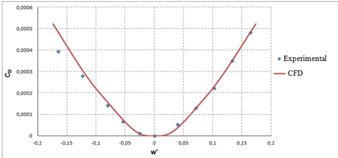
Figure 9: Variation of Drag Force Coefficients according to  $w'$
