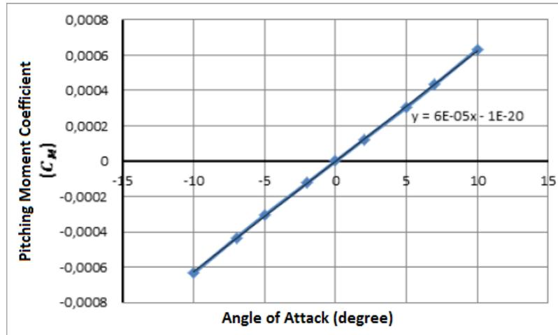
Figure 18: Pitching Moment Coefficient ( $C_M$ ) vs. Angle of Attack Graphic for 10 Knots Cruise Speed.
