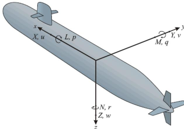
Figure 3: *Schematic of the cartesian coordinate system [6].*
