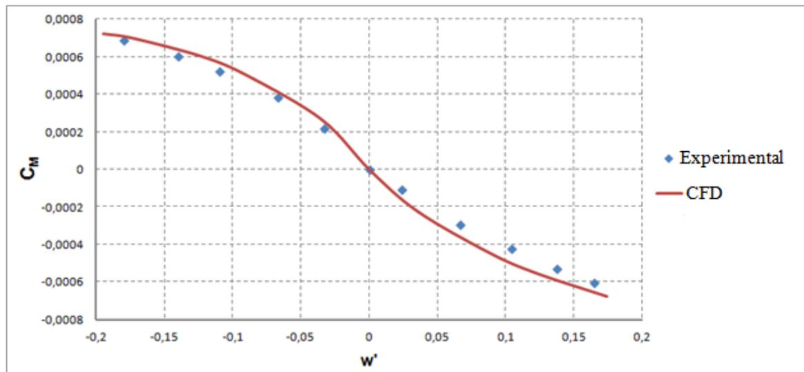
Figure 11: Variation of Pitch Moment Coefficients according to  $w'$
