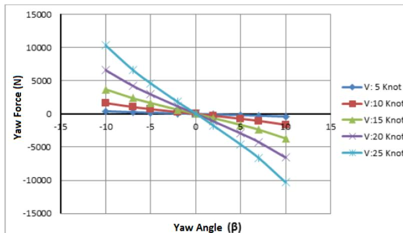
Figure 16: *Yaw Force vs. Sideslip Angle Graphic for Different Velocities.*
