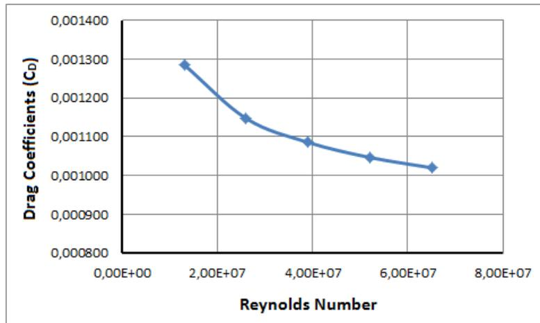
Figure 14: *Drag Coefficient vs. Re Number Graphic of Autosub.*
