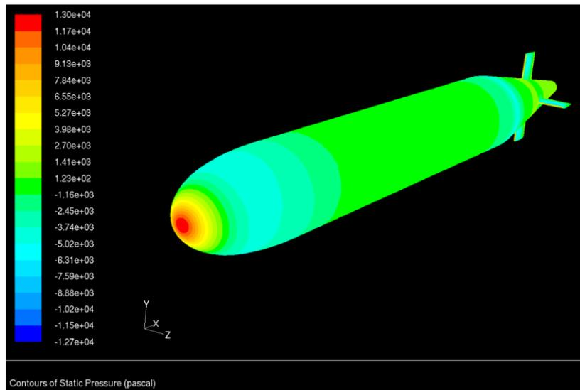
Figure 20: Pressure distributions over Autosub AUV in 10 knots.
