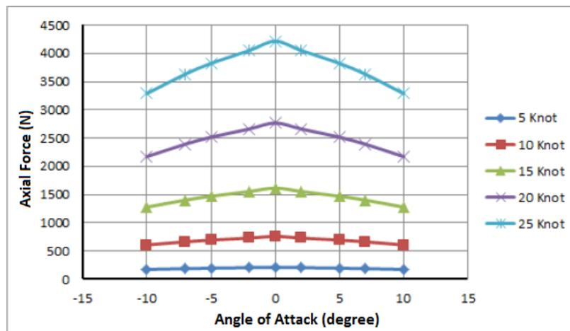
Figure 15: *Drag Forces - Angle of Attack Graphic for Different Velocities.*
