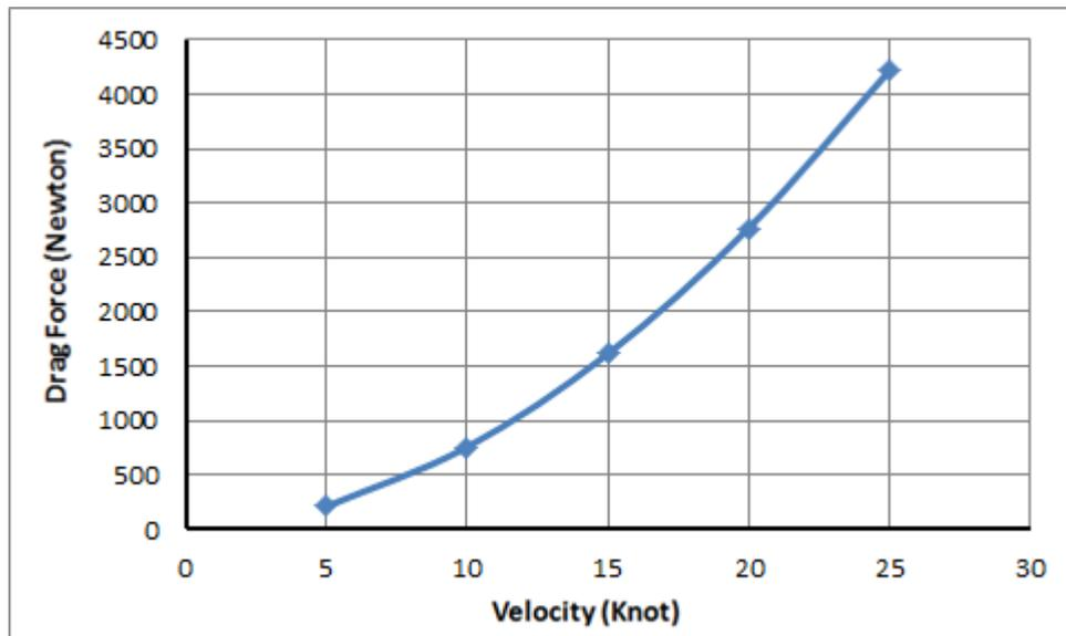
Figure 13: *Drag Forces vs. Velocity Graphics of Autosub.*
