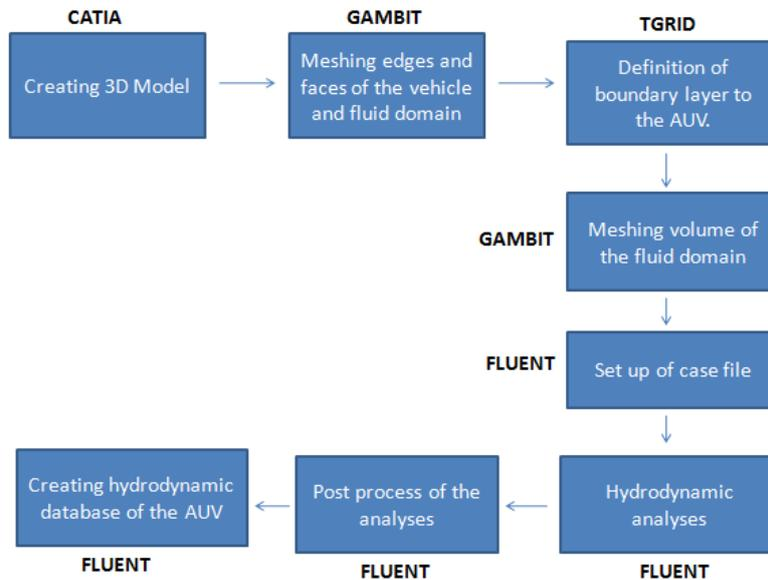
Figure.4: Flow chart of the hydrodynamic analysis process.
