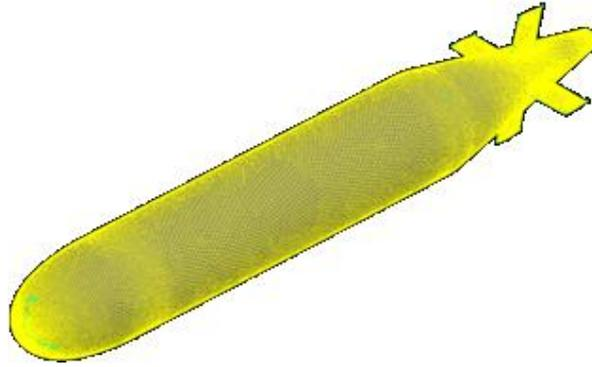
Figure 6: *Surface grids of Autosub AUV.*
