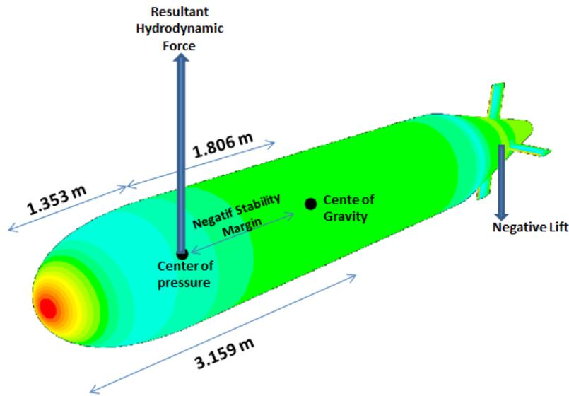
Figure 19: Center of Pressure and Center of Gravity Locations of Autosub.
