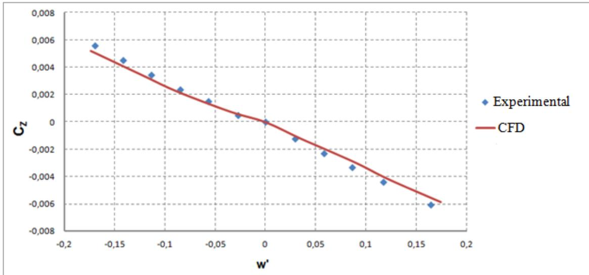
Figure 10: Variation of Surge Force Coefficients according to  $w'$
