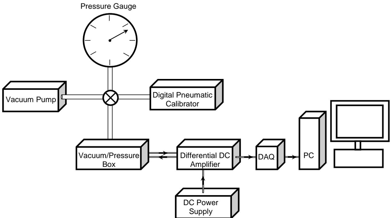
Figure 3: Schematic of the setup for calibration of pressure transducers
