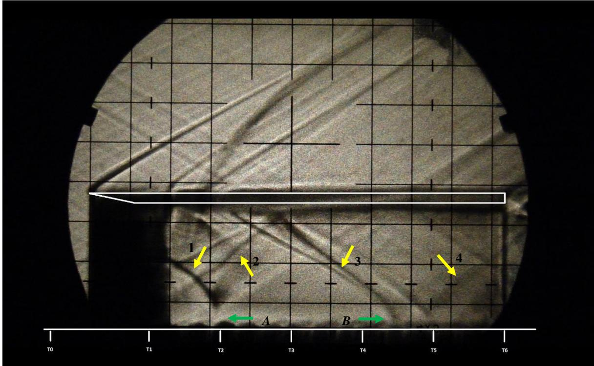
Figure 4: A sample schlieren image of flow in the inlet-isolator model at Mach 2.
