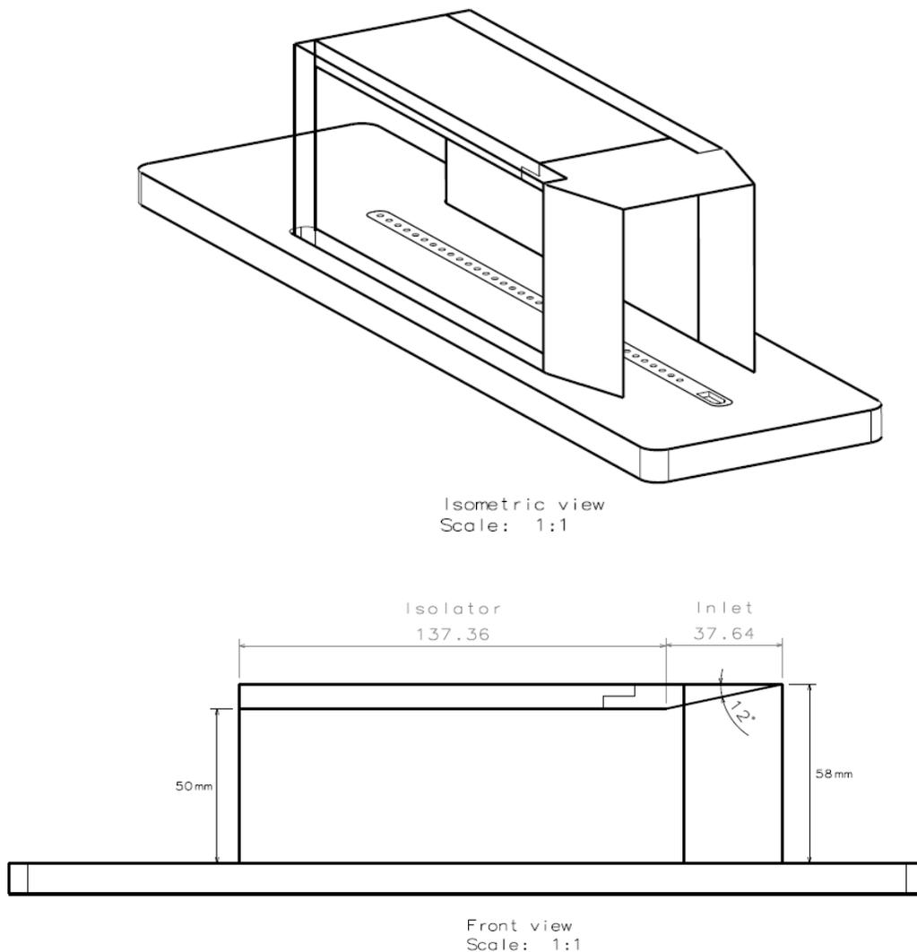
Figure 2: *Schematics of the inlet-isolator model instrumented for simultaneous optical and pressure measurements*
