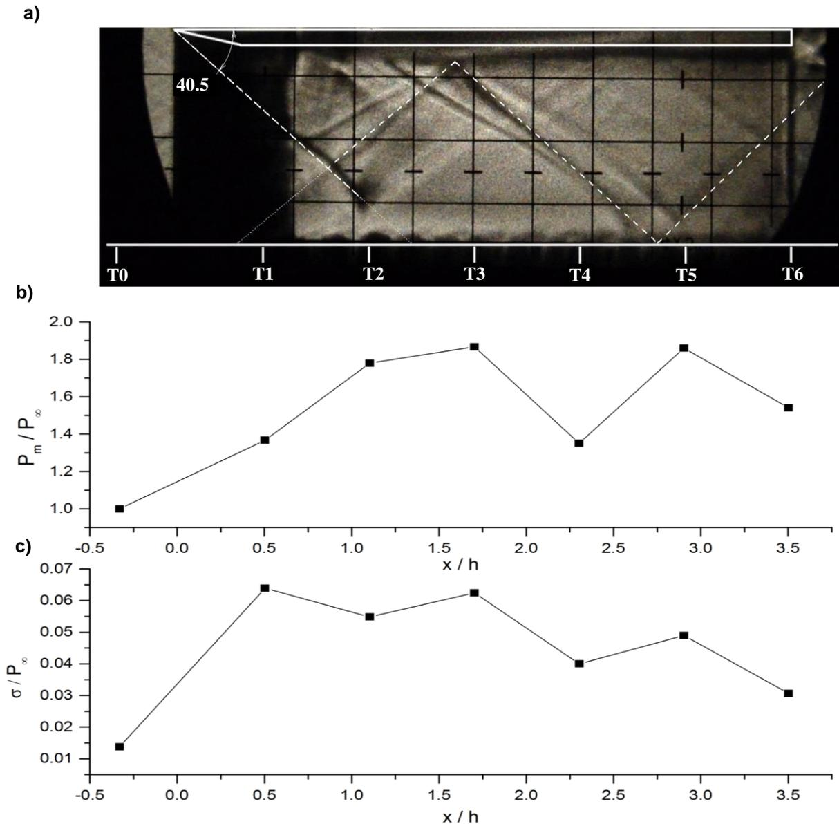
Figure 5: a) A schlieren image b) Mean pressure distribution along the inlet/isolator model
