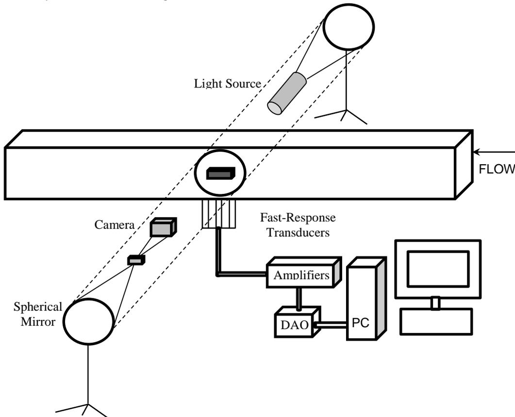
Figure 1: *Schematics of the model in the wind tunnel with schlieren imaging and fluctuating pressure measurements setup*
