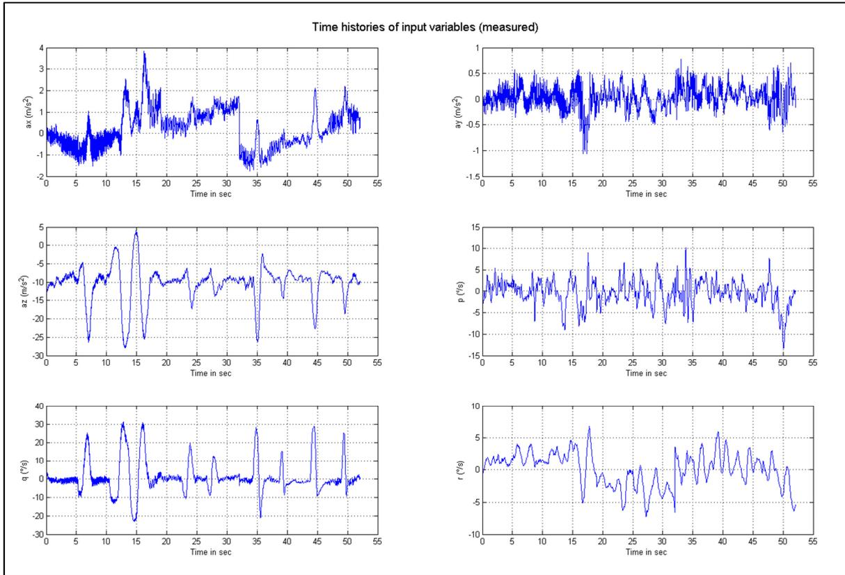
Figure 5: Time histories of input variables – Data compatibility check (logitudinal-directional motion)
