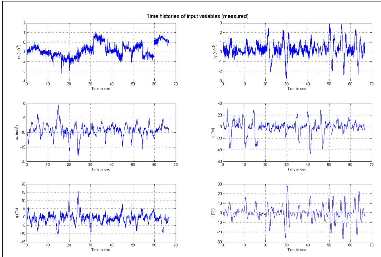
Figure 7: Time histories of input variables – Data compatibility check (lateral-directional motion)
