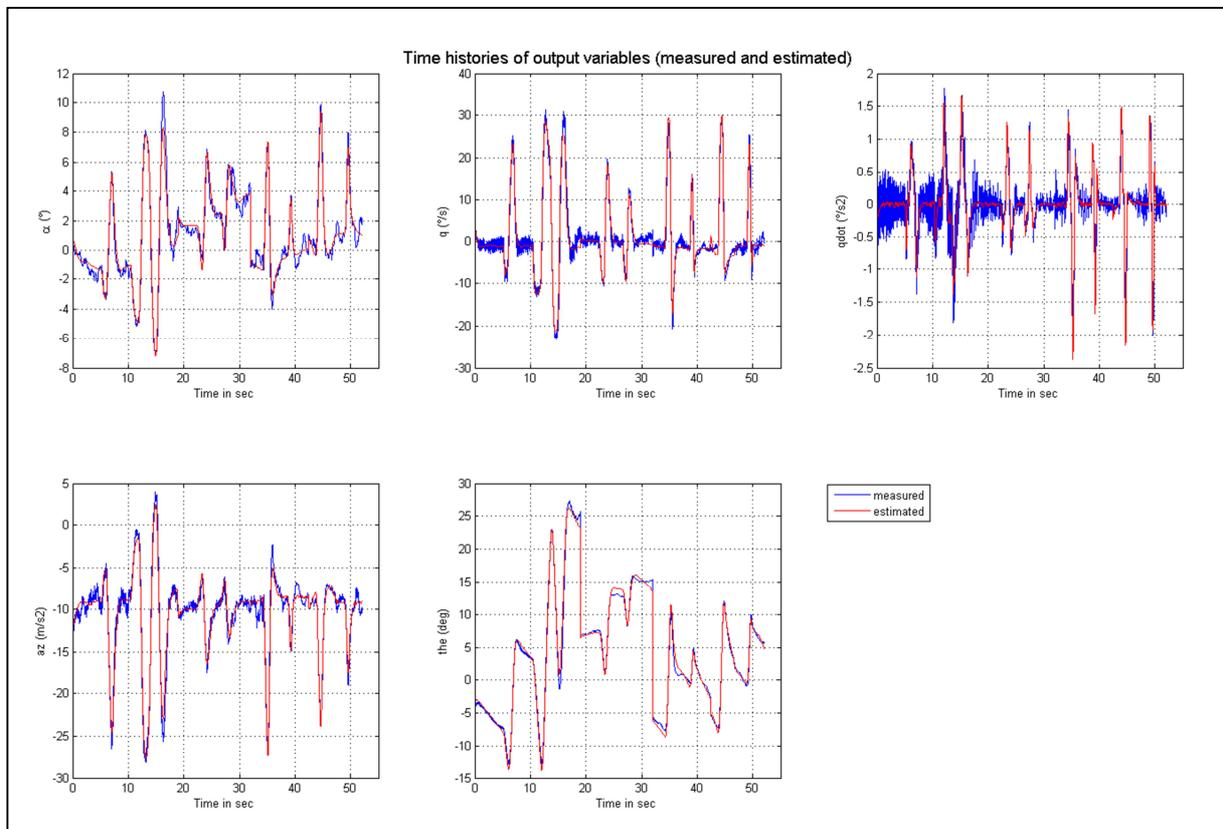
Figure 12: Time histories of output variables (measured and estimated) – Parameter estimation with output-error method (longitudinal-directional motion)
