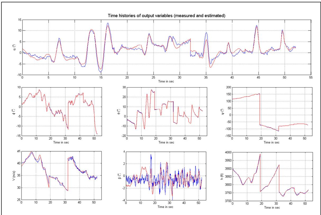
Figure 6: Time histories of output variables (measured and estimated) – Data compatibility check (logitudinal-directional motion)
