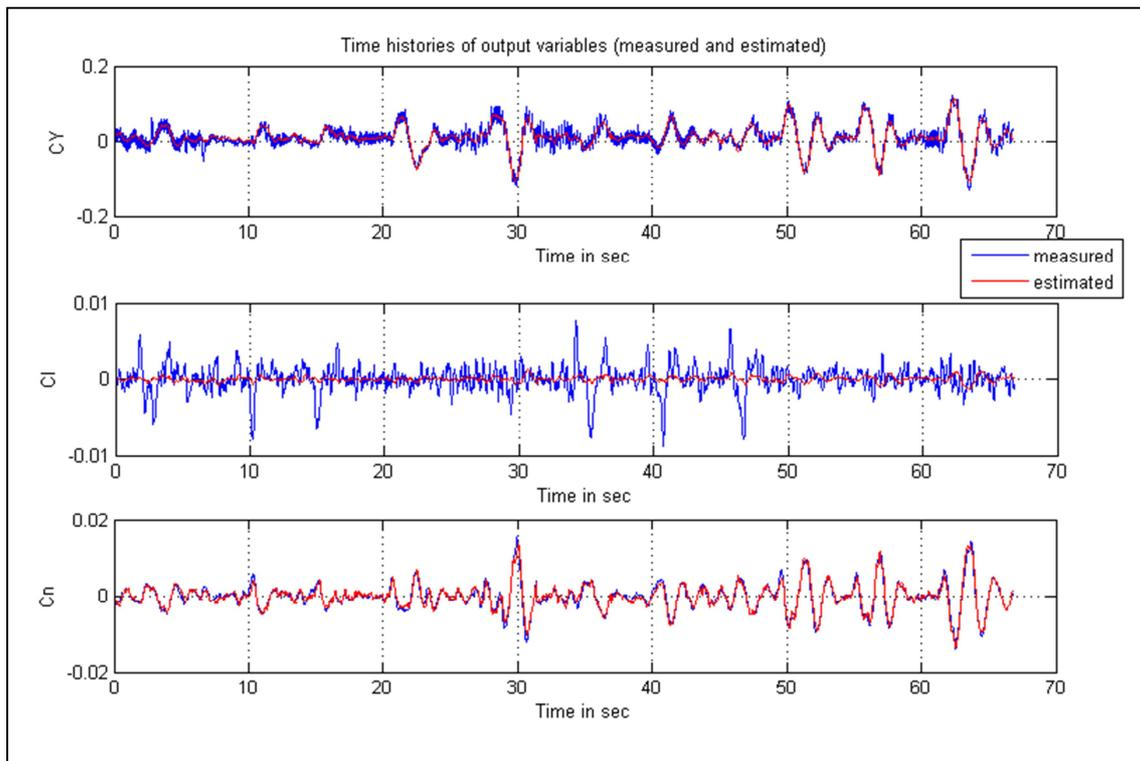
Figure 10: Time histories of output variables (measured and estimated) – Parameter estimation with equation-error method (lateral-directional motion)
