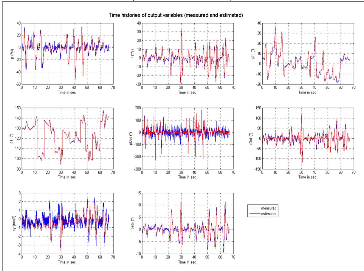
Figure 14: Time histories of output variables (measured and estimated) – Parameter estimation with output-error method (lateral-directional motion)
