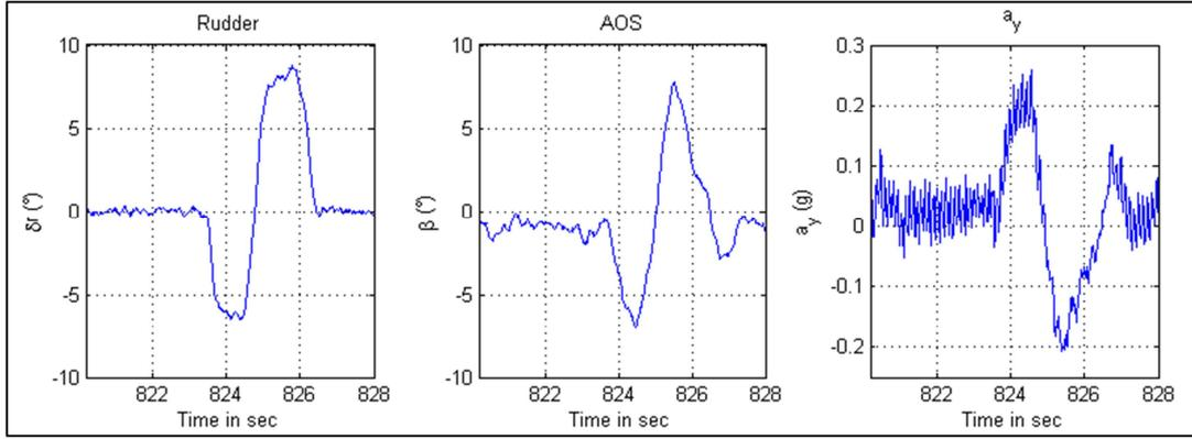
Figure 4: Rudder doublet input
