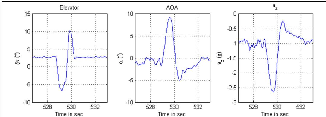
Figure 2: *Elevator doublet input*
