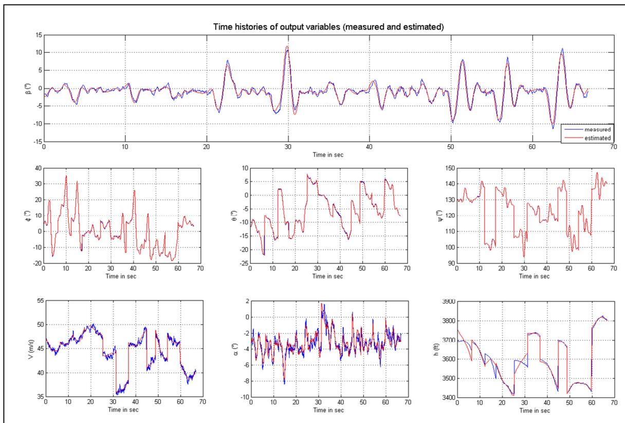
Figure 8: Time histories of output variables (measured and estimated) – Data compatibility check (lateral-directional motion)
