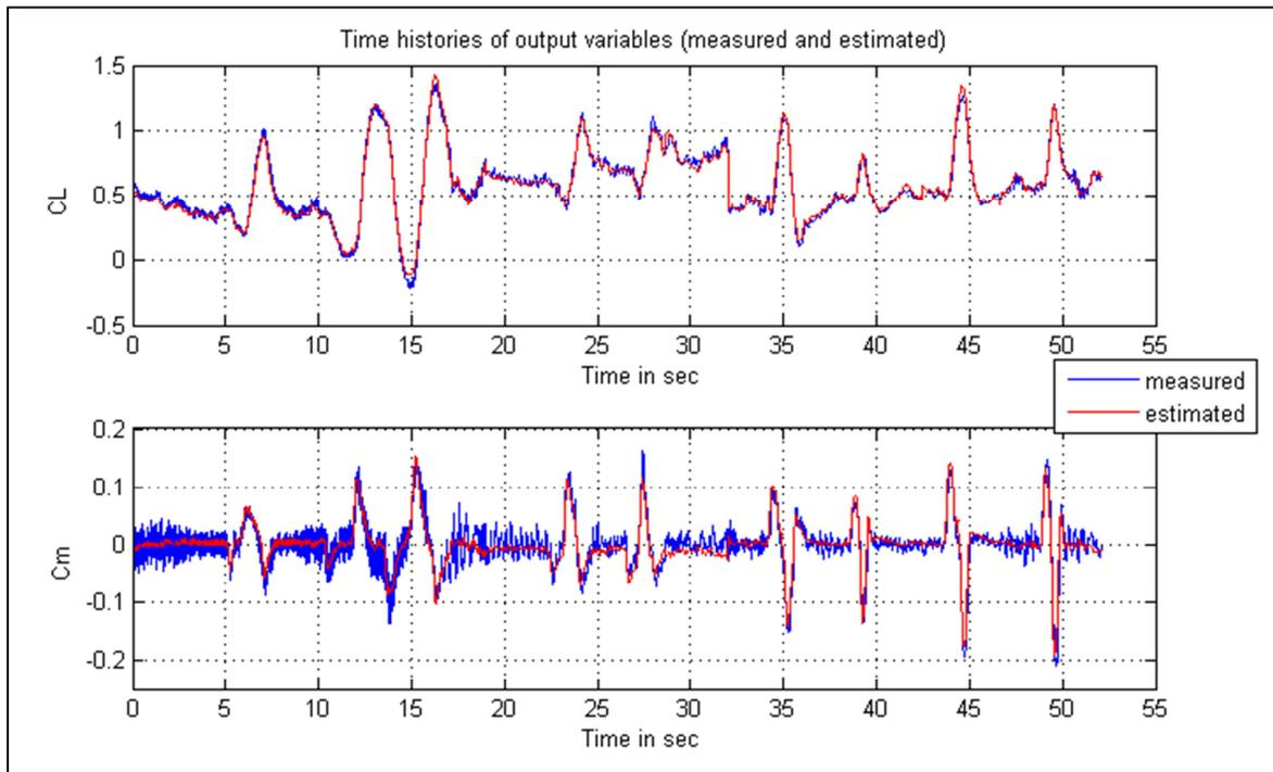
Figure 9: Time histories of output variables (measured and estimated) – Parameter estimation with equation-error method (longitudinal-directional motion)
