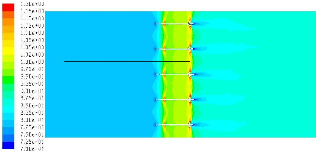
Figure 3b: *Mach number contours for estimated width-to-thickness ratio and free-stream Mach number of 0.85*
