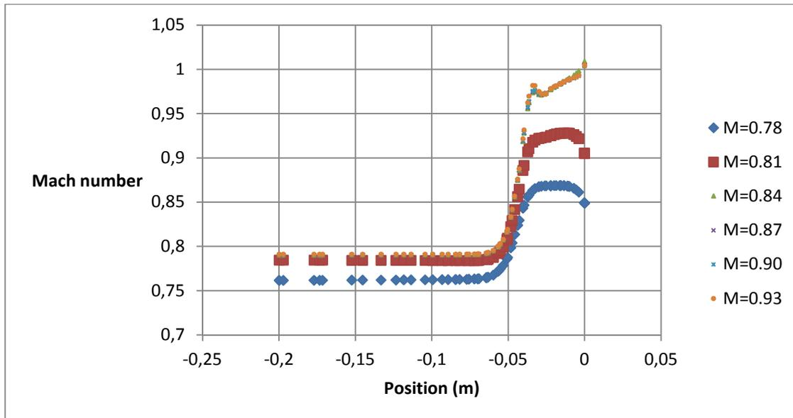
Figure 4: *Mach number along the centerline of model grid fin for different upstream boundary conditions*
