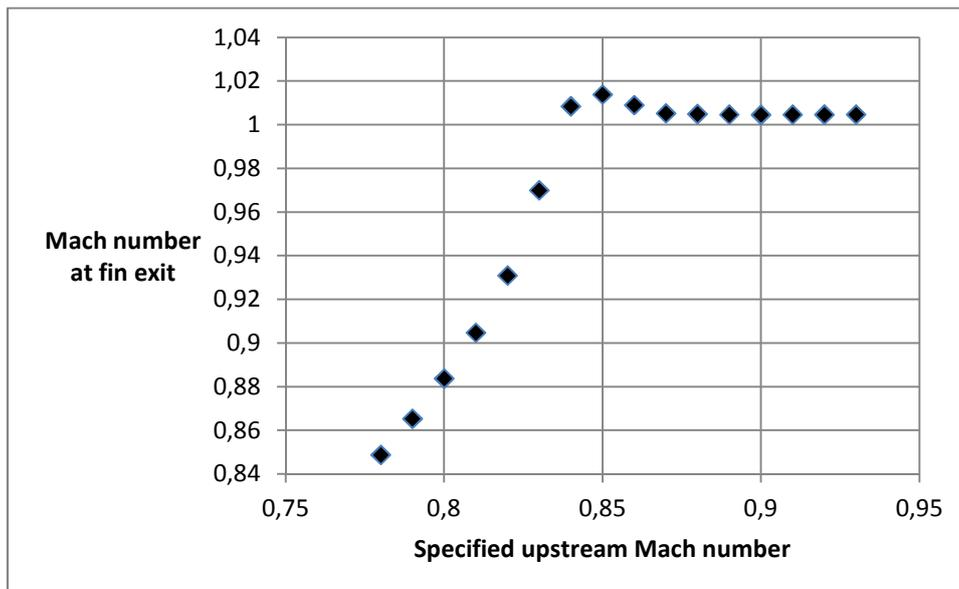
Figure 5: *Mach number at fin exit vs. specified upstream Mach number*
