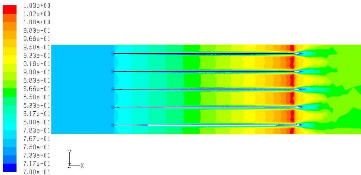
Figure 8: *Mach contour showing choking due to boundary layer formation*
