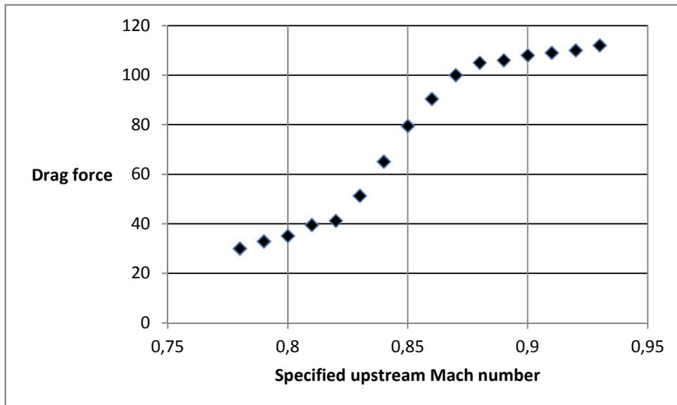
Figure 7: *Drag force vs. specified upstream Mach number*
