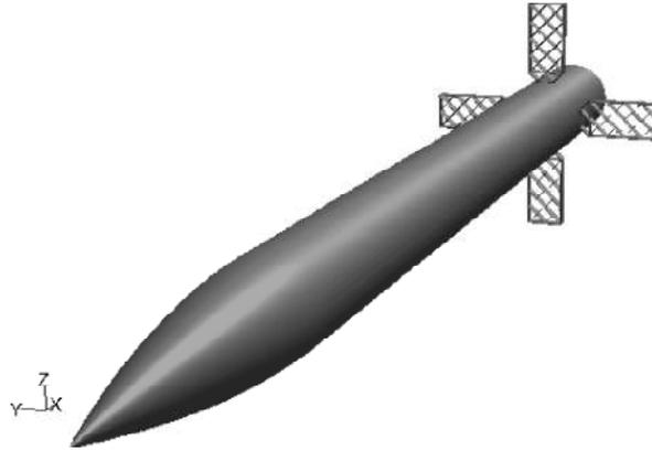
Figure 1: A schematic of grid fin control surfaces on a missile body [DeSpirito et al., 2001]
