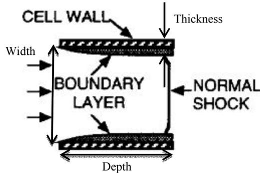
Figure 2: *Low transonic choking* [Washington and Miller, 1998]
