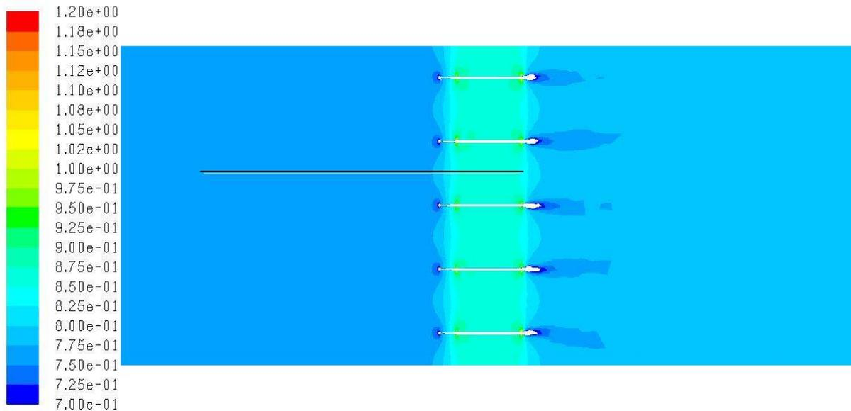
Figure 3a: *Mach number contours for estimated width-to-thickness ratio and free-stream Mach number of 0.78*
