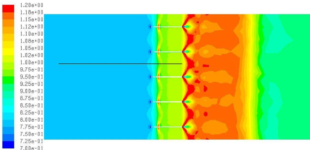
Figure 3c: *Mach number contours for estimated width-to-thickness ratio and free-stream Mach number of 0.90*
