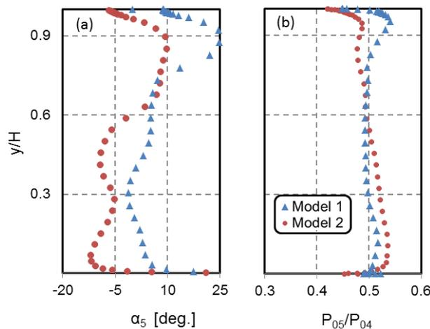
Figure 12. Stage outlet radial distributions a) absolute swirl angle, b) Non-dimensional total pressure
