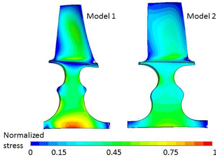
Figure 10. Rotor stress levels
