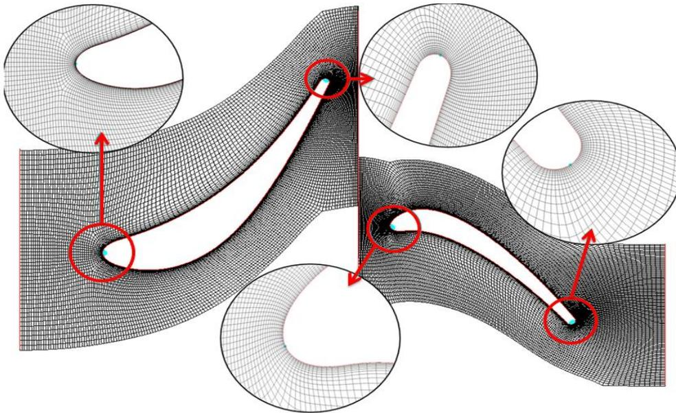
Figure 3. Computational domain and mesh topology
