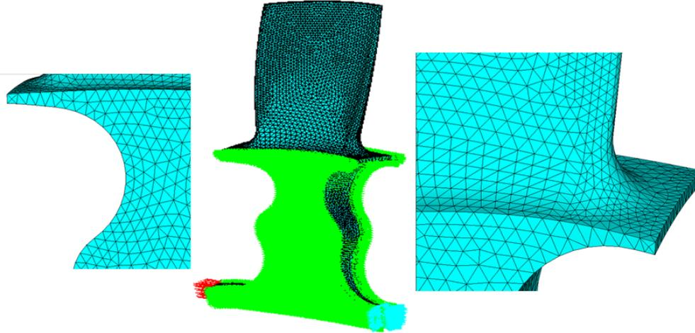
Figure 5. FEM model of the rotor
