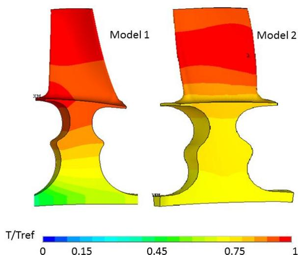
Figure 6. Temperature distribution of the both model
