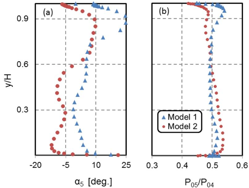
Figure 8. Stage outlet radial distributions a) absolute swirl angle, b) Non-dimensional total pressure
