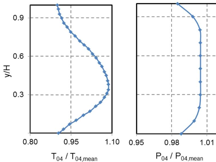
Figure 4. Turbine inlet total temperature and pressure profiles
