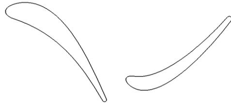
Figure 2. Model 2 mid span vane and blade
