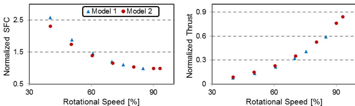
Figure 9. Engine test results of both turbines a) fuel consumptions b) thrust rating
