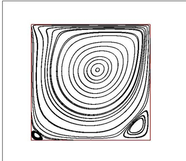
Figure 3 Computed streamlines inside the cavity for  $Re = 400$ .
