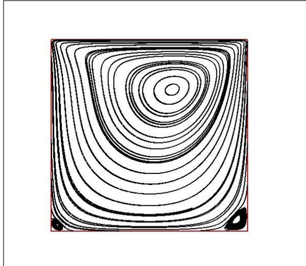
Figure 2 Computed streamlines inside the cavity for  $Re = 100$ .
