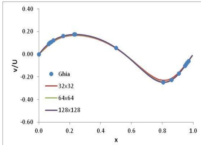
Figure 5 Comparison of velocity components in x and y directions, respectively, with the results from [Ghia, U., Ghia, K.N., and Shin, C.T. 1982], for  $Re = 100$ .
