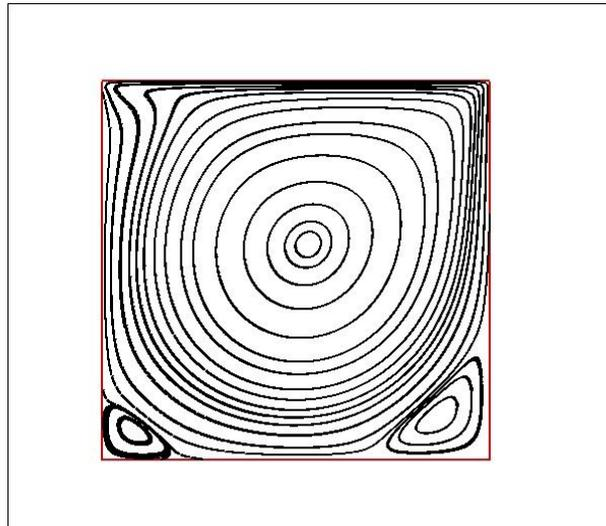
Figure 4 Computed streamlines inside the cavity for  $Re = 1000$ .
