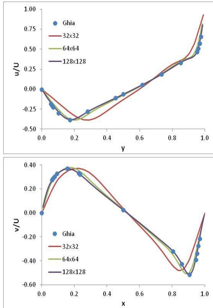
Figure 7 Comparison of velocity components in x and y directions, respectively, with the results from [Ghia, U., Ghia, K.N., and Shin, C.T. 1982], for Re=1000.
