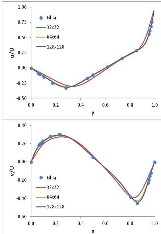
Figure 6 Comparison of velocity components in x and y directions, respectively, with the results from [Ghia, U., Ghia, K.N., and Shin, C.T. 1982], for  $Re = 400$ .
