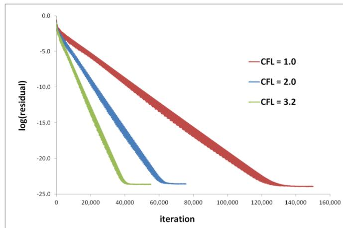
Figure 8 Comparison of convergence history for different CFL numbers at Re=400
