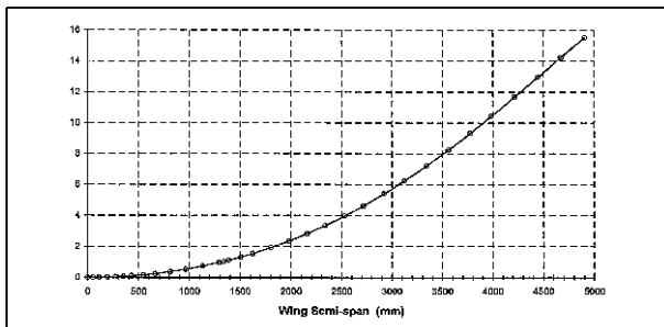
Figure 7: 1 st bending mode, wing 2 , (15.7 Hz)
