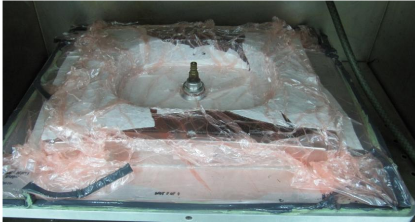
Fig. 25: Compaction and heating process of preform
