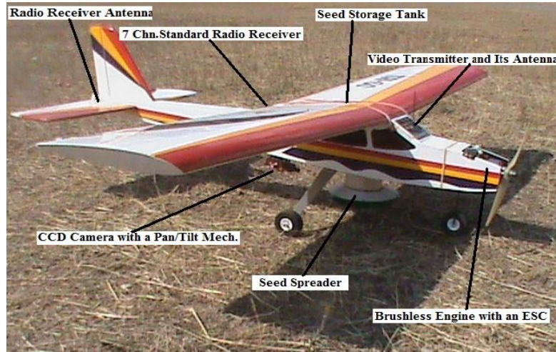
Figure 4: The UAV developed for reforestation of Lebanon cedar
