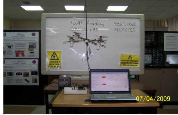
Figure 4: Experimental platform of altitude control for a Quadrotor
